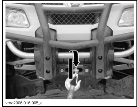
TYPICAL — FRONT TIE-DOWN POINT LOCATION
