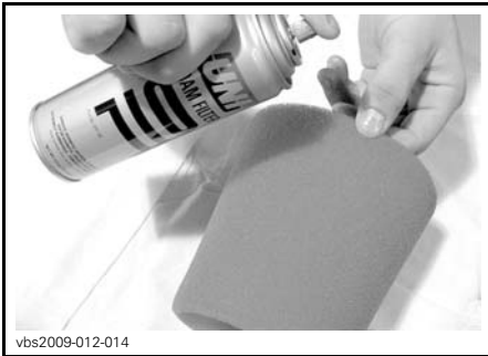
TYPICAL - OIL FOAM FILTER ELEMENT
