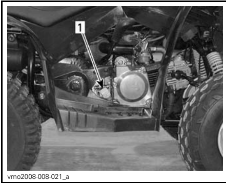
TYPICAL — RH SIDE OF ENGINE 1. Dipstick
