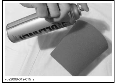
TYPICAL - SPRAY FOAM ELEMENT INSIDE AND OUT
