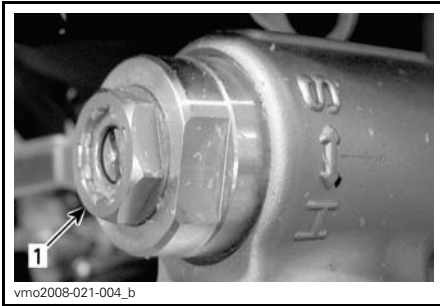
1. High speed compression adjuster (17 mm wrench)
