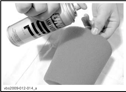
TYPICAL - OIL THE FOAM FILTER ELEMENT
