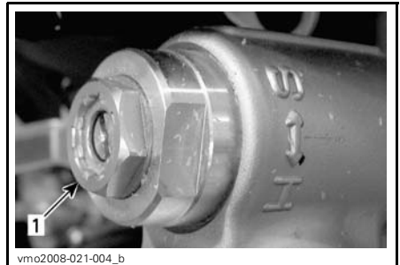
TYPICAL 1. High speed compression adjuster
