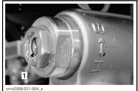
TYPICAL 1. Compression adjuster (flat screwdriver)
