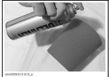
TYPICAL - SPRAY THE FOAM ELEMENT
