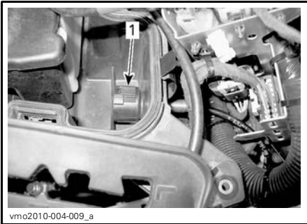
1. ACS compressor air filter
