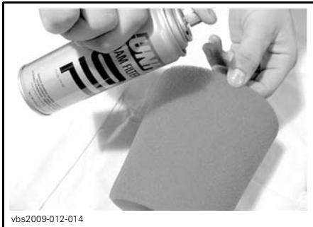
TYPICAL - OIL THE FOAM FILTER ELEMENT
