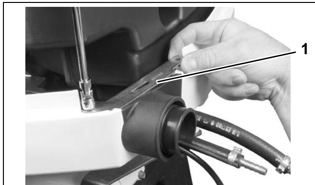
1. Grommet retaining bracket
