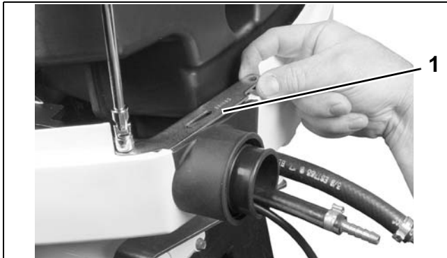
1. Grommet retaining bracket
