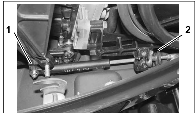
1. Shift cable retainer clip and washer 2. Shift cable trunnion
