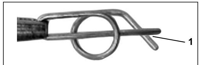
Locked Retainer Clip 1. Angled section behind straight section DP0817A
