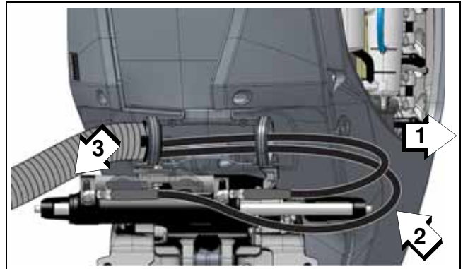
Starboard Entry Shown 1. Outboard turned OPPOSITE hose entry 2. Inspect hydraulic hoses NOT kinked 3. Inspect steering cylinder NOT contacting rigging hose 009913-1
