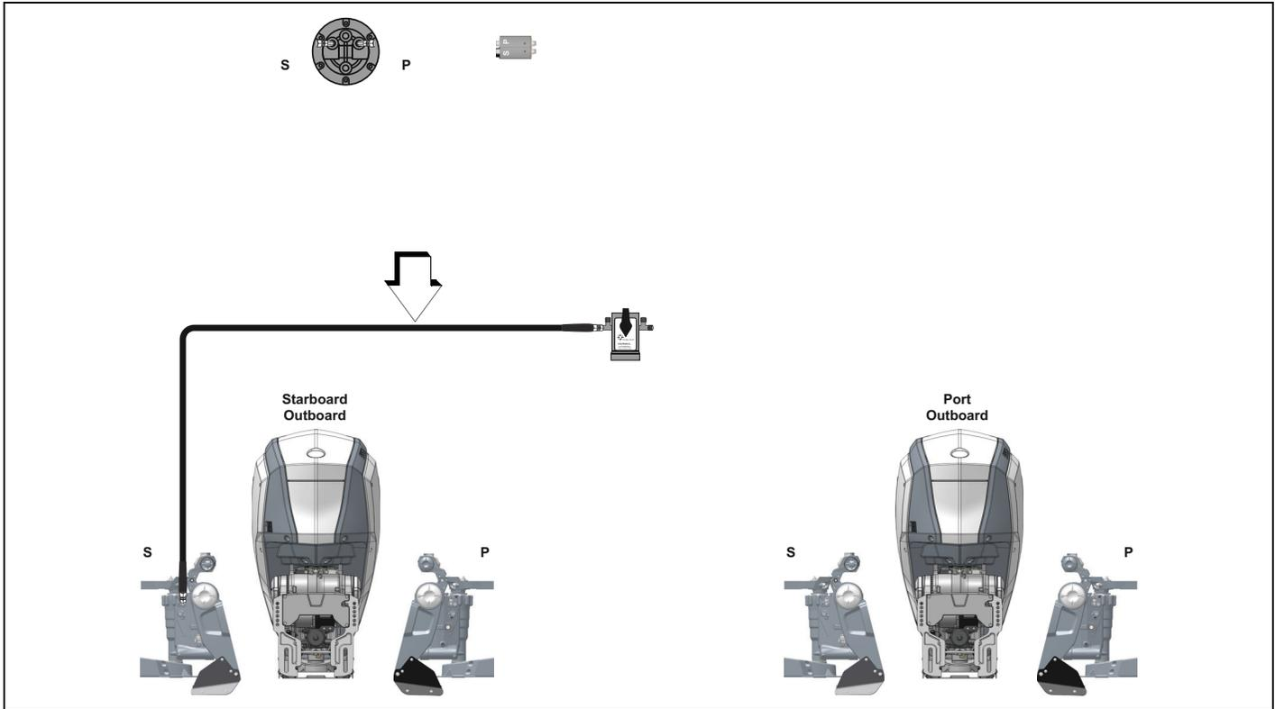
Connect a 1000 PSI hydraulic hose from the Steering Pressure Sensor to the port side of the starboard engine.
