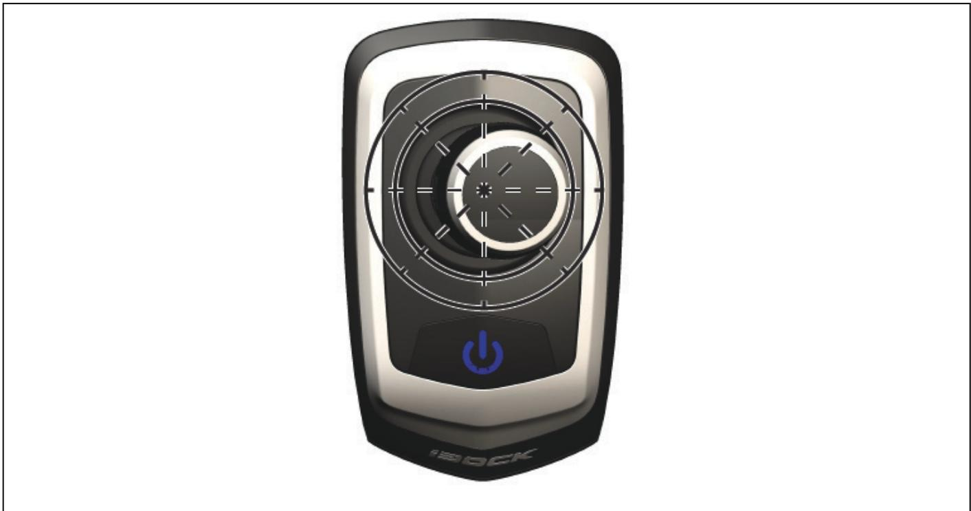
While holding the joystick right, use the *Increase Throttle* and *Decrease Throttle* buttons to set the desired starboard speed.
