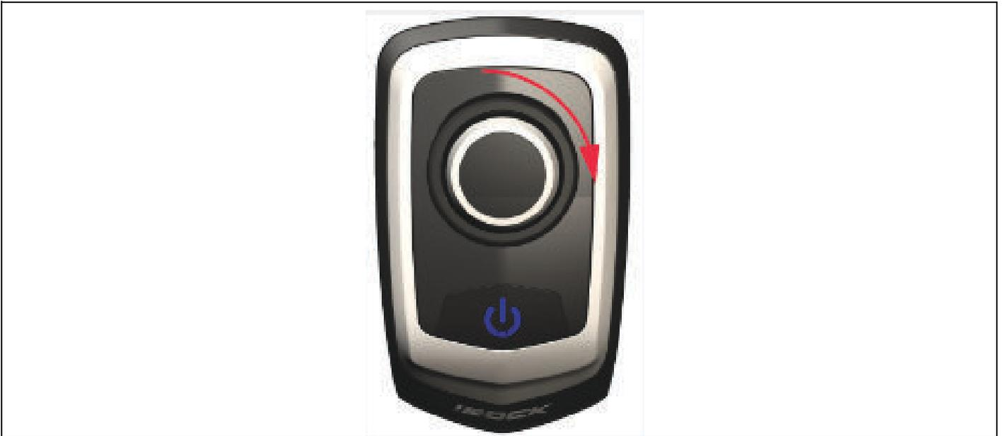
When the joystick is turned clockwise, the port engine will provide forward thrust while the starboard engine will provide reverse thrust to spin the vessel starboard.
