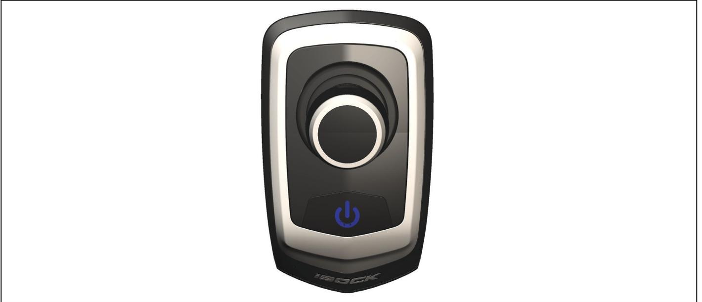
When the joystick is pushed aft, both the port and starboard engines will provide reverse thrust to move the vessel aft.
