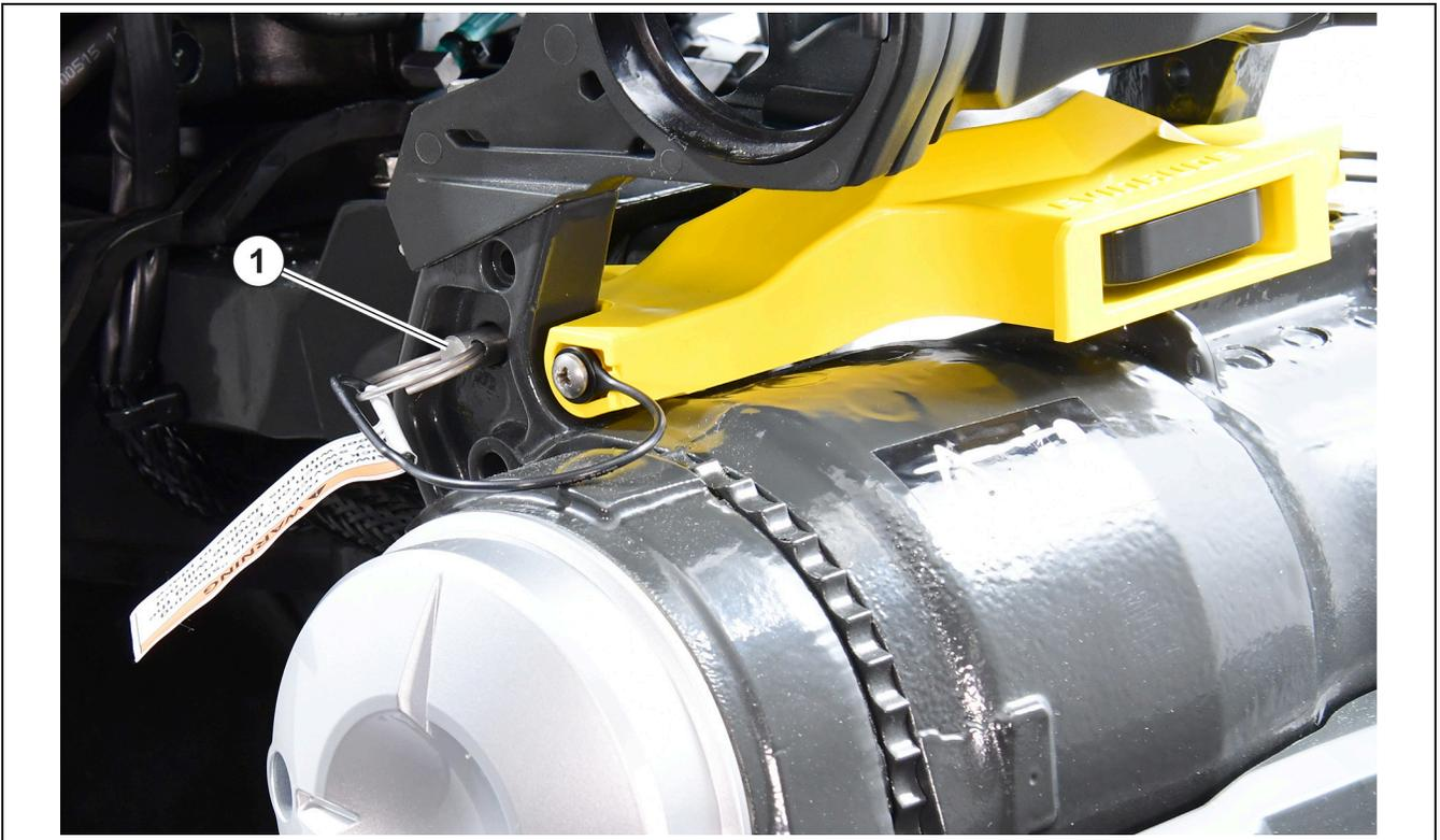
1. Quick release pin (STARBOARD side shown)
