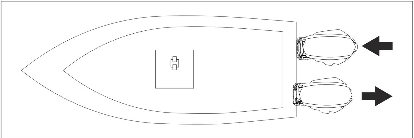
To increase the movement, twist the joystick further counterclockwise.
