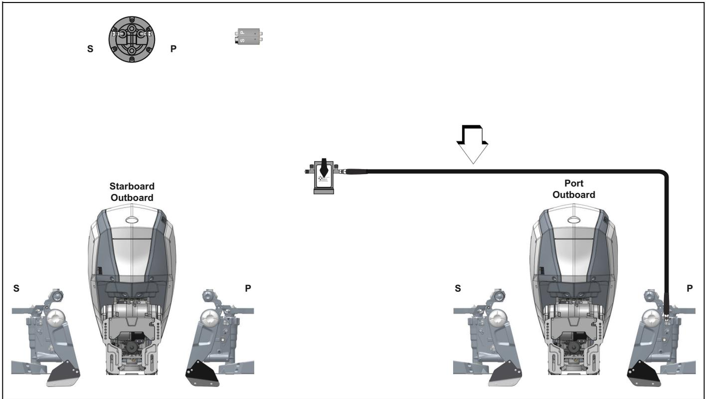
Connect a high pressure (rated for 3000 PSI) hydraulic hose from the Alignment Valve to the starboard side of the port engine. Torque the hose fittings to 13 ft. lbs. (18 N·m).
