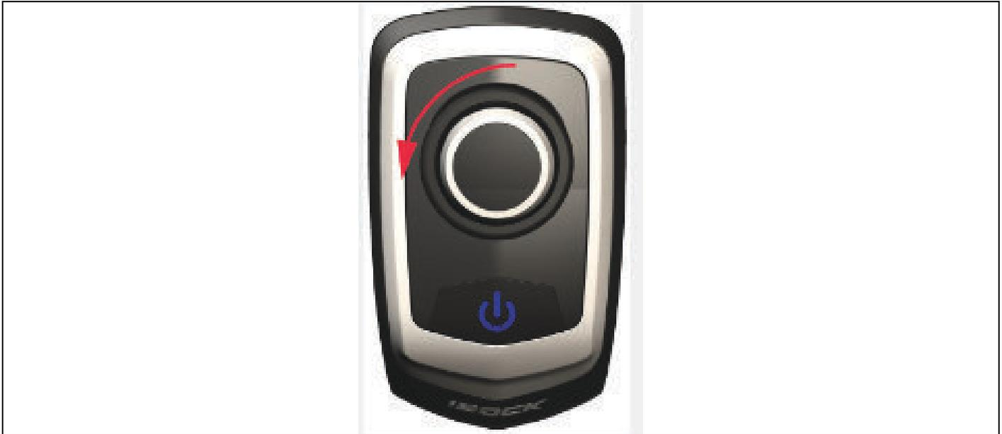
When the joystick is turned counterclockwise, the port engine will provide reverse thrust and the starboard engine will provide forward thrust to spin the boat to port.
