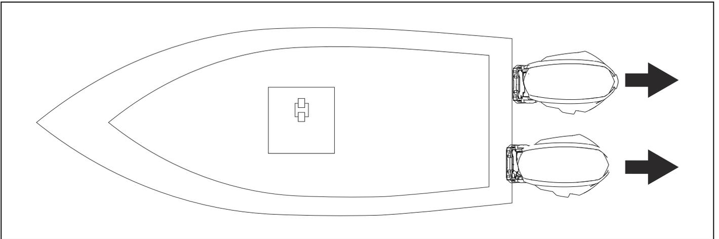
To increase the movement, push the joystick harder (past the detent) in the aft direction.
