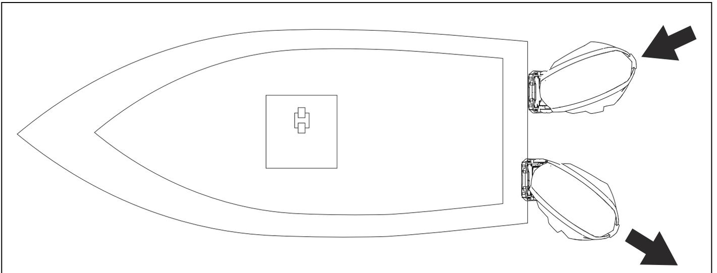
To increase the movement, push the joystick harder (past the detent) in the port/left direction.
