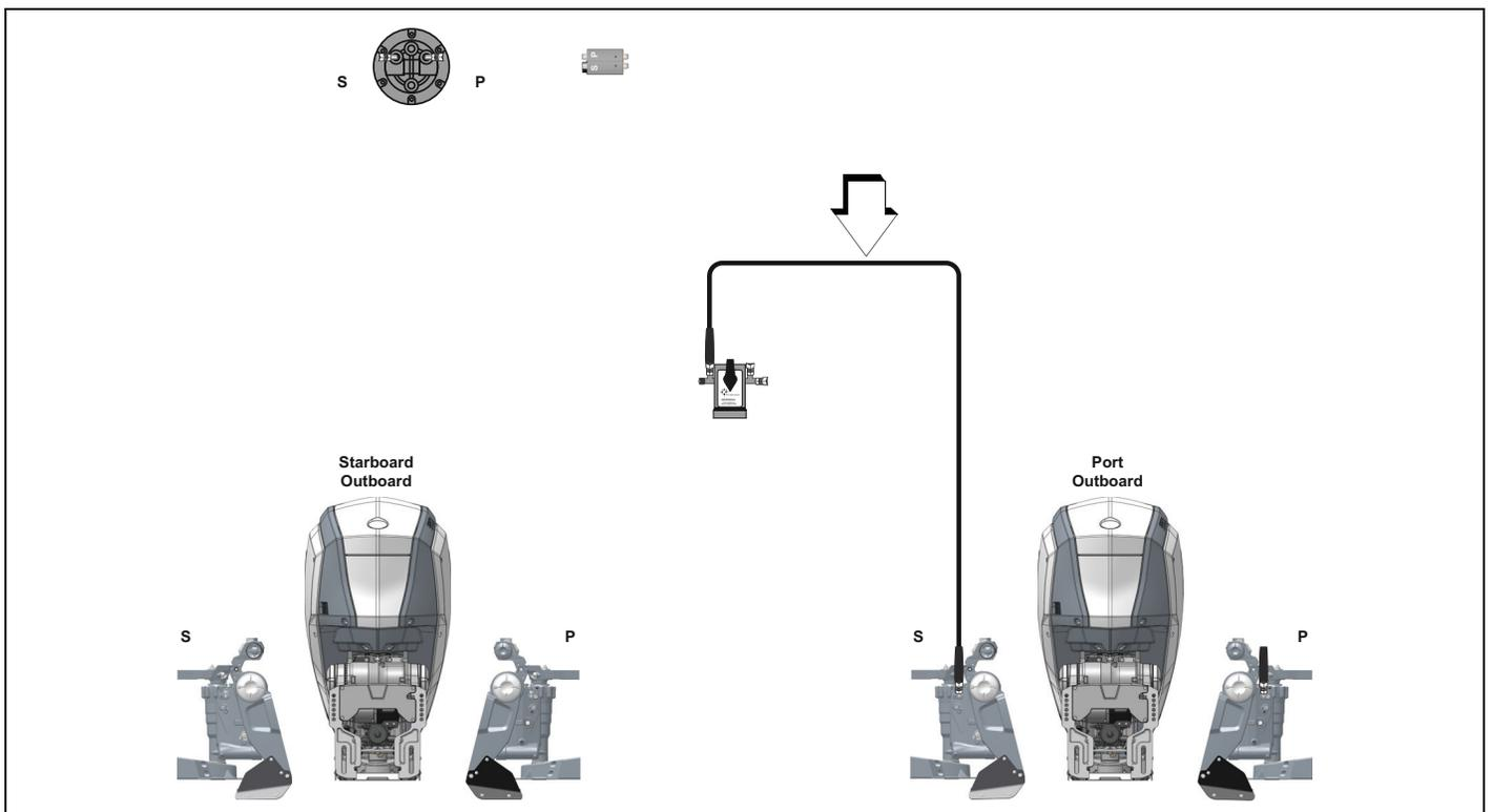
Connect a high pressure (rated for 3000 PSI) hydraulic hose from the Alignment Valve to the starboard side of the starboard engine. Torque the hose fittings to 13 ft. lbs. (18 N·m).
