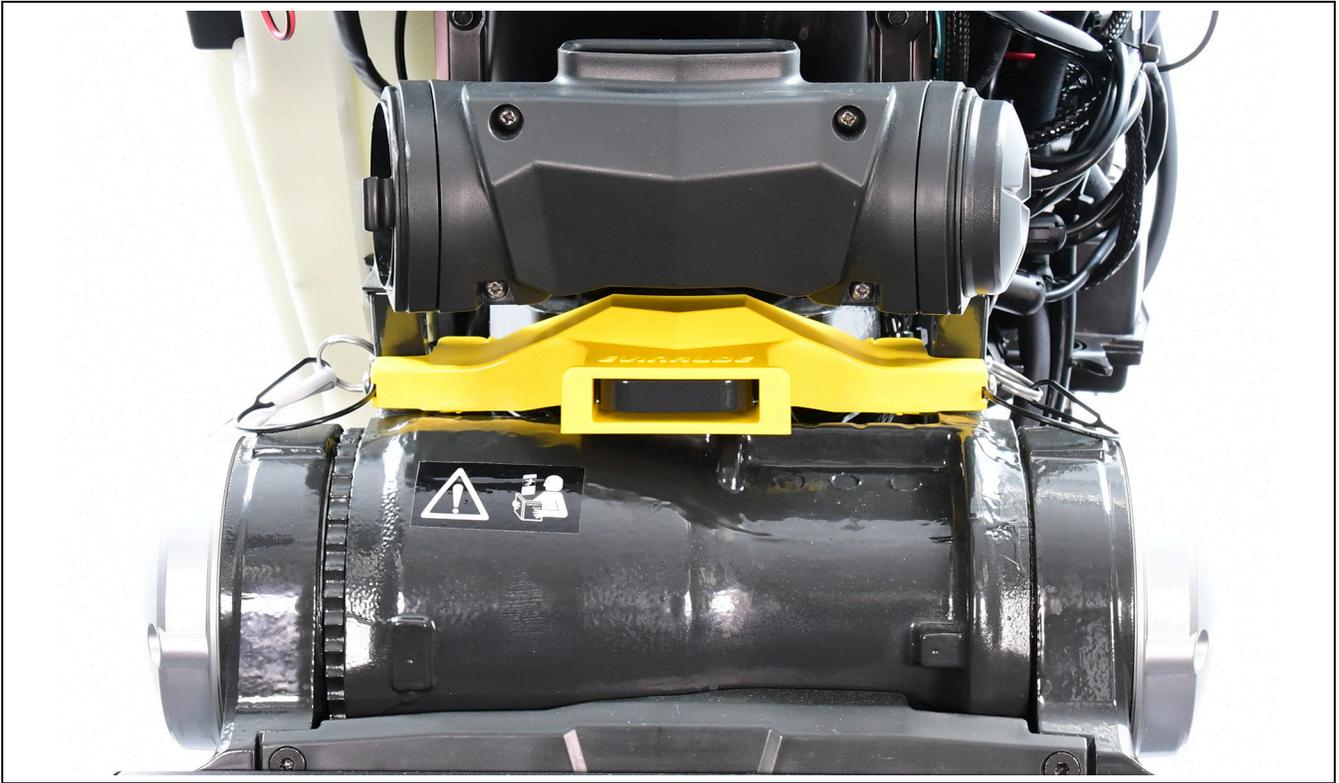
Install two quick release pins through the holes on each side of the stern bracket.
