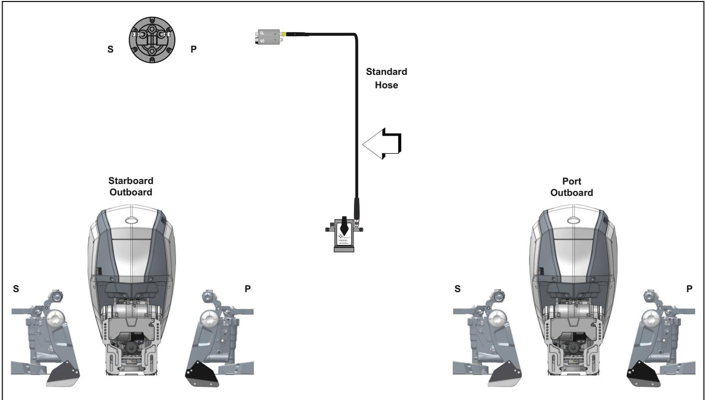
Connect a 1000 PSI hydraulic hose from the Alignment Valve to the port side of the port engine.
