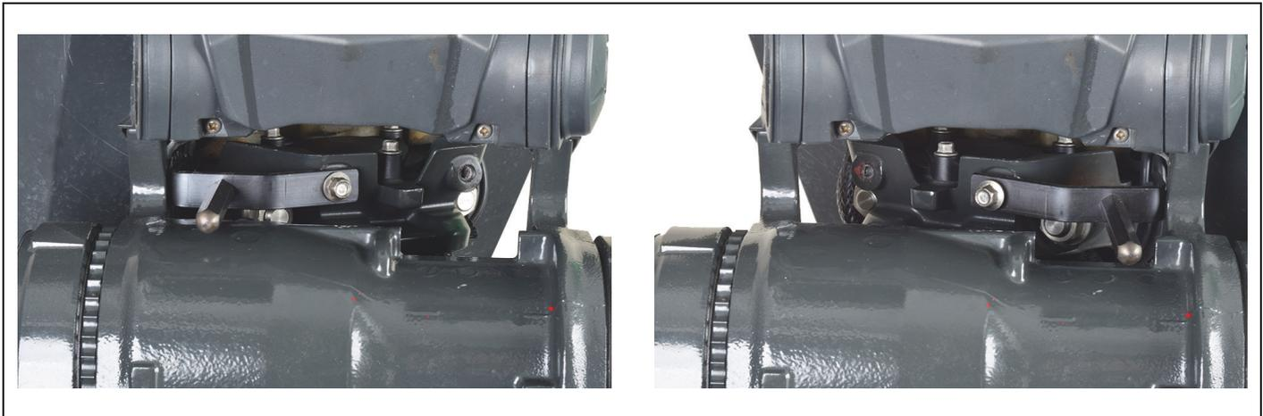
STEERING LOCK TOOL, P/N 357717, INSTALLED
