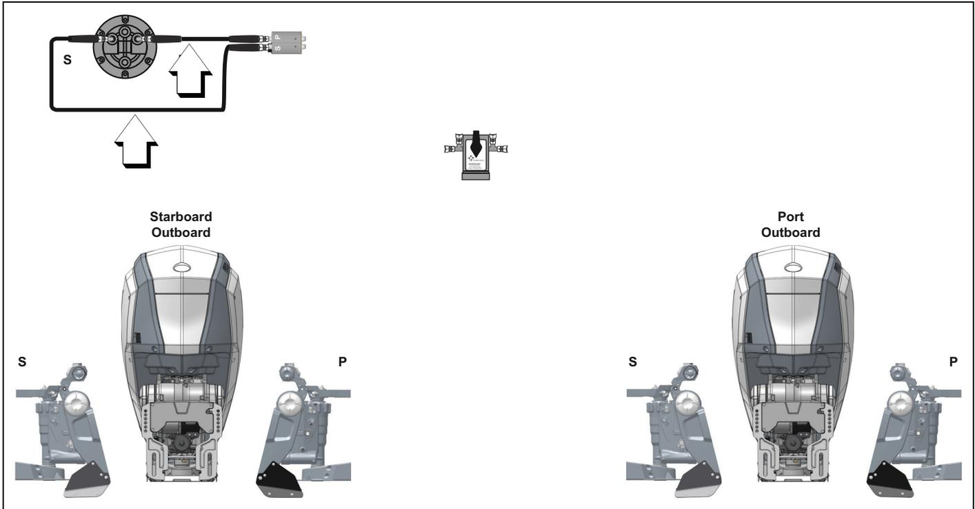
Connect a 1000 PSI hydraulic hose from the Pressure Sensor Assembly to the Alignment Valve.
