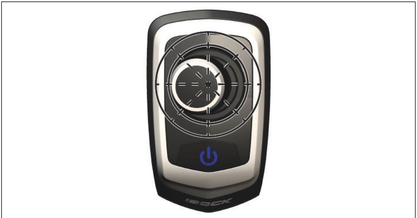
While holding the joystick left, use the *Increase throttle* and *Decrease throttle* buttons to set the desired port speed.
