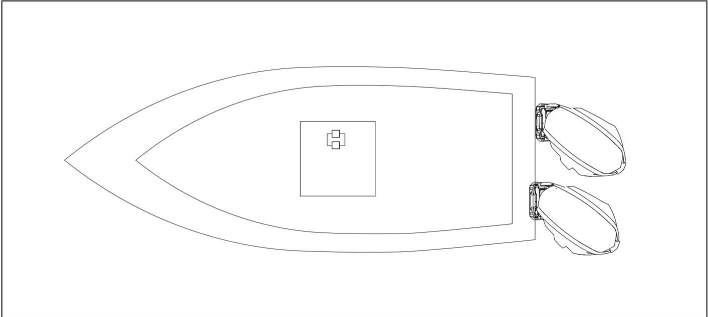
Install one Steering Lock Tool, P/N 357717, onto each outboard to hold the outboards in a full port turn.
