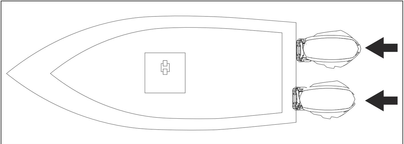
To increase the movement, push the joystick harder (past the detent) in the forward direction.
