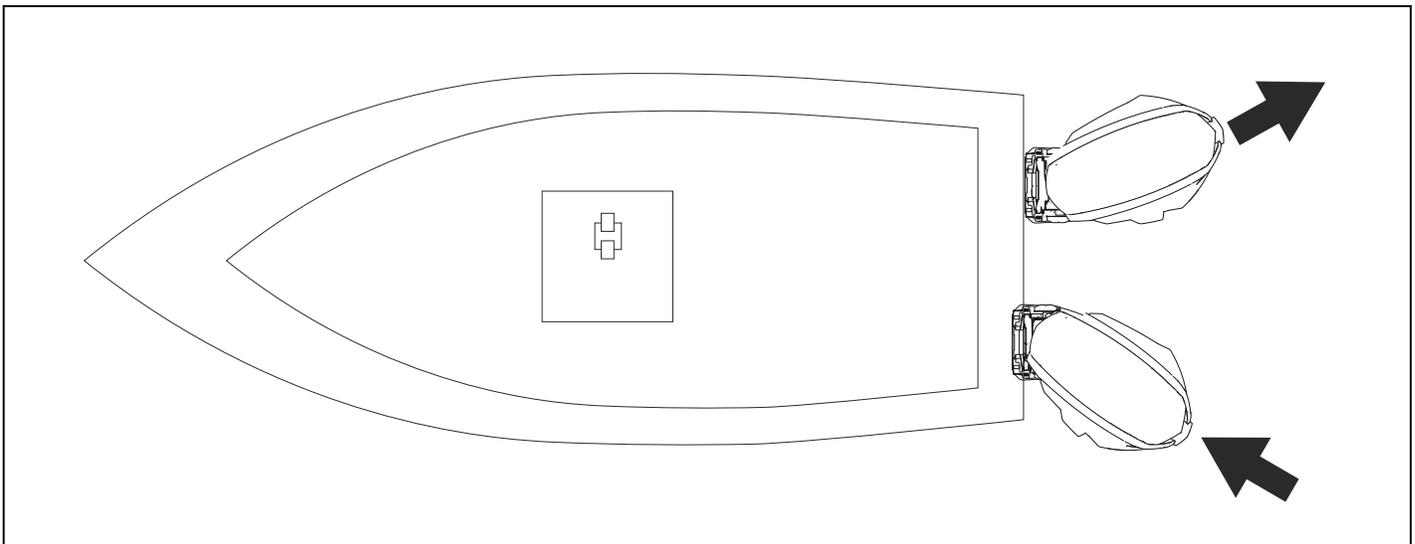
To increase the movement, push the joystick harder (past the detent) in the starboard/right direction.
