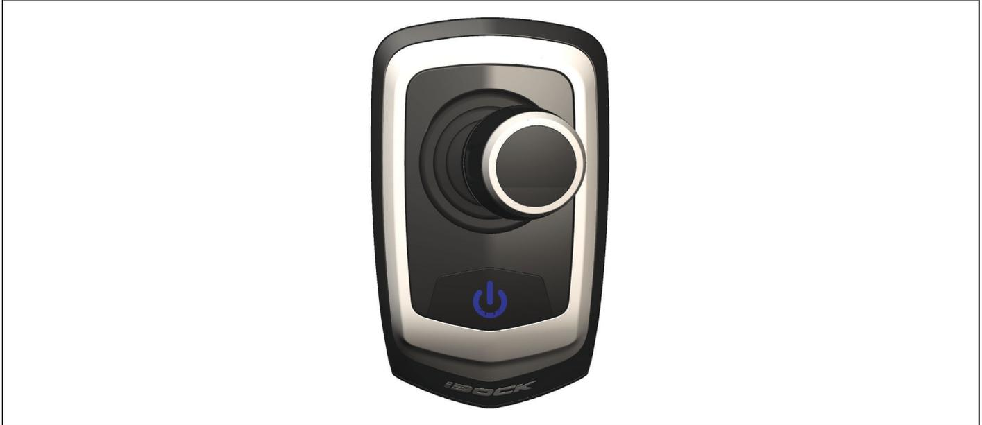
When the joystick is pushed to starboard, the port engine will provide reverse thrust while the starboard engine will provide forward thrust to walk the boat starboard.
