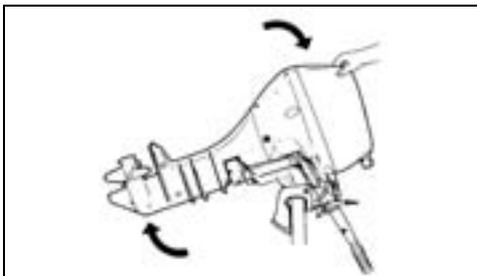
Slowly, lower motor until shallow-water drive bracket rests against angle adjusting rod.
