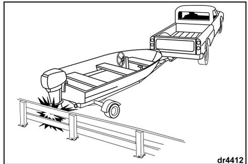
If you hit any object, stop immediately and examine the engine for loosening of attaching hardware and clamp screws, if equipped. Inspect for damage to swivel and stern brackets, steering components, and components in the area of impact. Also, examine the boat for structural damage. Tighten any loosened hardware. If the collision occurred in the water, proceed slowly to harbor. Before boating again, have your Dealer thoroughly inspect all components.
