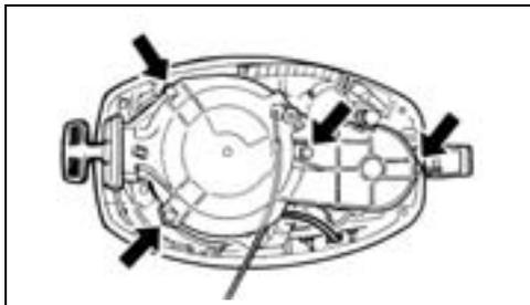
Tie a knot in one end of the emergency starter cord. Thread the small bar from the tools kit halfway through one knot so it forms a handle.
