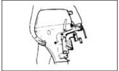
The resulting position of the anti-ventilation plate must be 0 to 1 in. (0 to 25 mm) below the boat's bottom.
