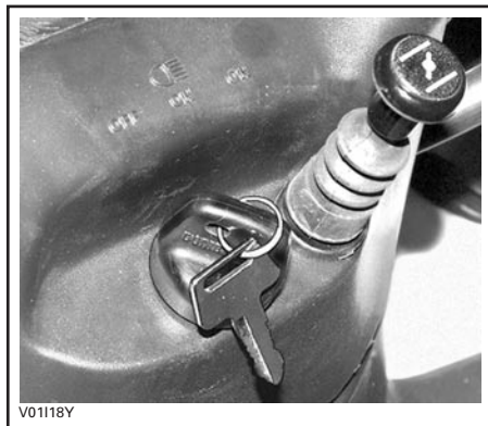
CHOKE LEVER IN THE FULL CHOKE POSITION
