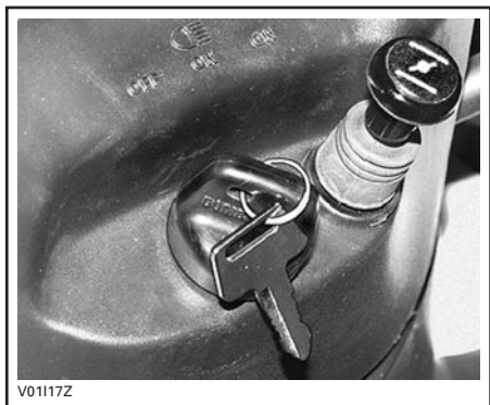
CHOKE KNOB LEVER IN THE OFF POSITION
