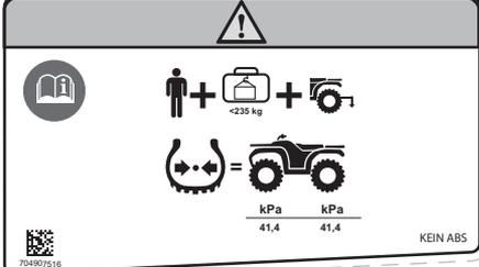
Warning sign for non-ABS models. It features a central warning triangle with an exclamation mark and a book icon. To the left, a person and a bag icon are shown with a weight limit of <math>< 235 \text{ kg}</math>. Below, a tire pressure diagram shows front and rear tire pressures in kPa: both 41.4. The text 'KEIN ABS' is in the bottom right corner. A QR code is in the bottom left corner.
