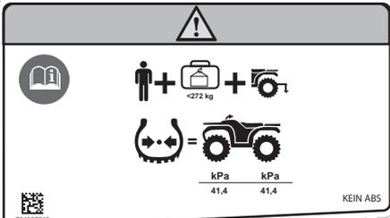
Warning sign for non-ABS models. It features a central warning triangle with an exclamation mark and a book icon. To the left, a person and a bag icon are shown with a weight limit of <math>< 272 \text{ kg}</math>. Below, a tire pressure diagram shows front and rear tire pressures in kPa: both 41.4. The text 'KEIN ABS' is in the bottom right corner. A QR code is in the bottom left corner.
