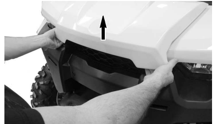
LIFTING FRONT SERVICE COVER EDGE.
