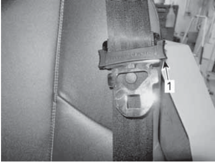
TYPICAL - LOCKED POSITION
