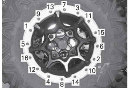
TYPICAL - TIGHTENING SEQUENCE
