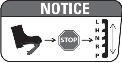
A diagram illustrating the shifting procedure. On the left, a black boot is shown stepping on a foot brake. An arrow points to a black octagonal sign with the word 'STOP' in white. Another arrow points to a vertical shift lever. The lever has five positions labeled from top to bottom: L, H, N, R, and P. A double-headed vertical arrow is positioned to the right of the lever, indicating its range of motion.
