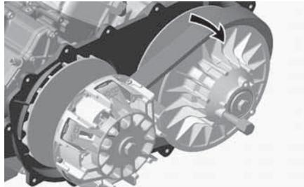
**Installing the Drive Belt**
