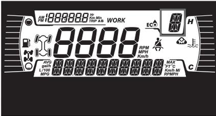
This display shows gear position of gearbox:
