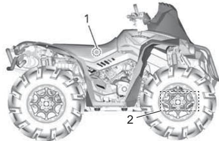
1. VIN Label - On the frame under the seat
