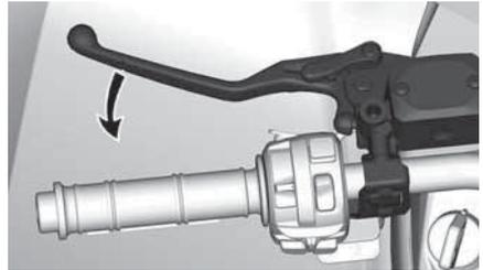
Braking effect is proportional to the force applied on the lever.
