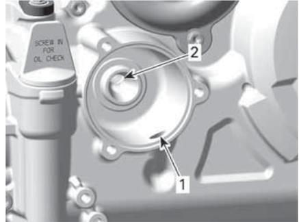
1. Inlet bore from the oil pump to the oil filter
