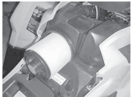
AIR FILTER REMOVAL
