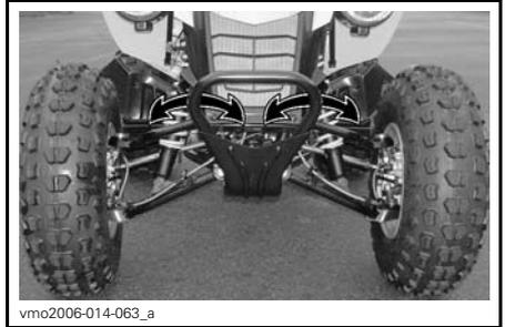
*EMPLACEMENT DES COURROIES DU PARE-CHOCS AVANT*
