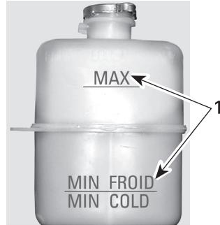
1. Level between marks when engine is cold B00067
