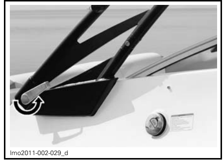
STARBOARD SIDE - TURN HANDLE 3/4 TURN COUNTERCLOCKWISE TO LOCK
