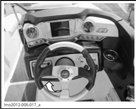
CIRCUIT BREAKER PANEL LOCATION
