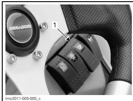
1. Bilge pump switch
