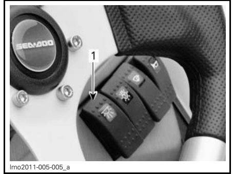
1. Deck light switch
