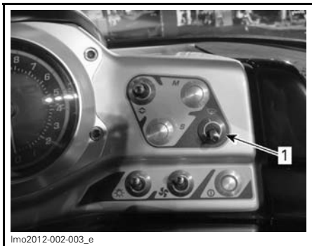
1. Bilge pump switch
