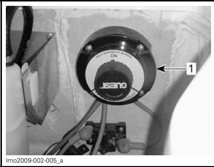
TYPICAL — MAIN BATTERY CUT-OFF SWITCH
