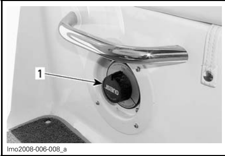
1. Main battery cut-off switch
