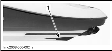
TYPICAL — BOTH SIDES 1. Intake grate
