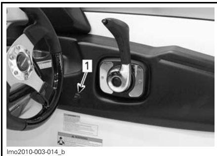
1. Emergency engine stop switch
