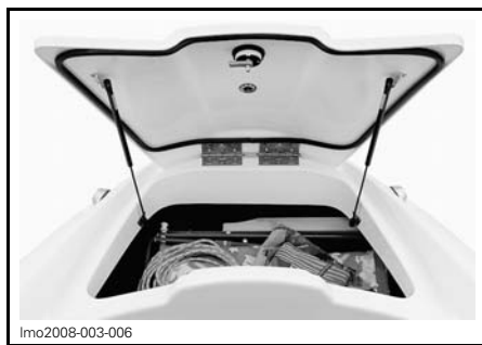
TYPICAL — BOW STORAGE COMPARTMENT
