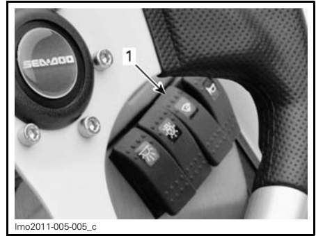
1. Bilge pump switch
