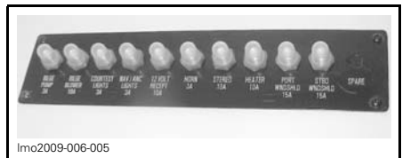
CIRCUIT BREAKER PANEL
