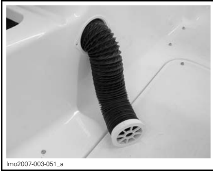
HEATING DUCT STRETCHED
