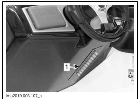
1. Circuit breaker panel location
