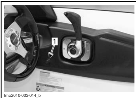
1. Emergency engine stop switch
