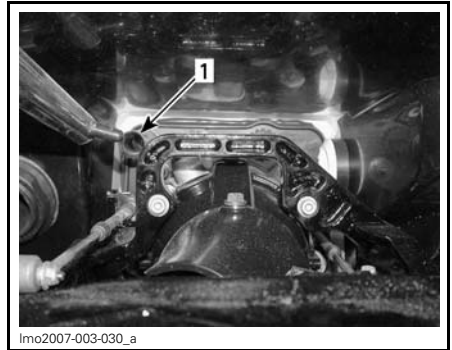
TYPICAL 1. Flushing connector
