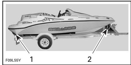
TYPICAL 1. Stern eyelet 2. Bow eyelet
