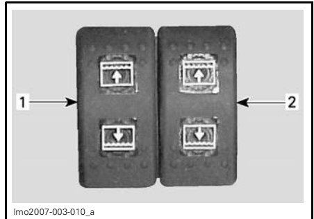
BALLAST BAG SWITCHES
