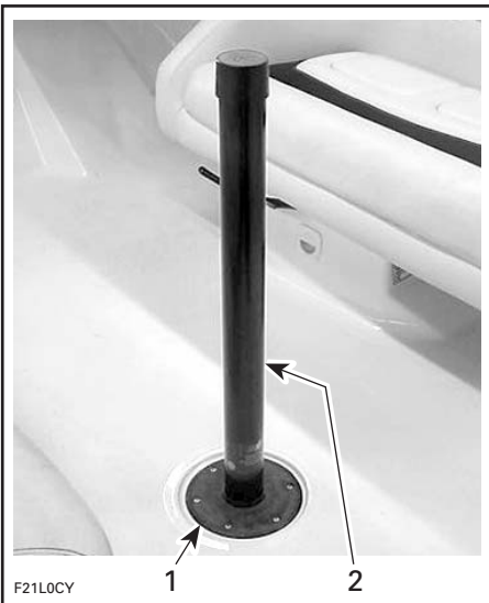
TYPICAL — POST IN POSITION 1. Floor receptacle 2. Table post
