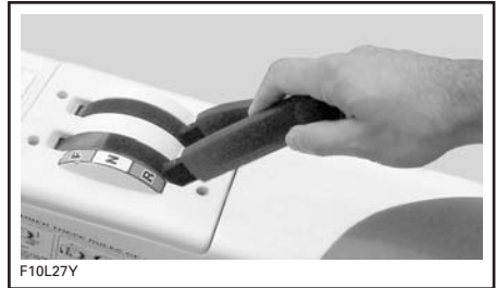
TYPICAL — SHIFTER LEVER IN REVERSE POSITION
