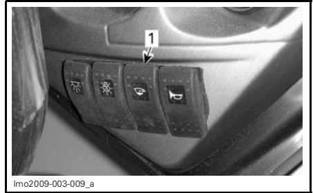
1. Bilge pump switch
