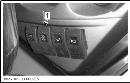
1. Navigation lights switch
