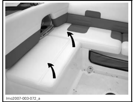
TYPICAL — PULL ON CUSHION TO RELEASE
