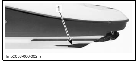
TYPICAL — BOTH SIDES 1. Jet pump water intakes
