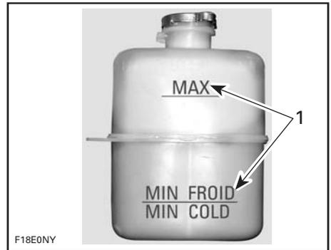
1. Level between marks when engine is cold
