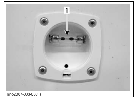
1. Pull and remove bulb
