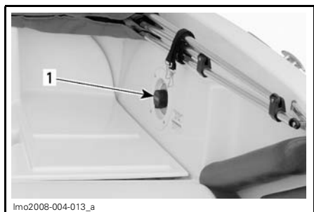
1. Main battery cut-off switch
