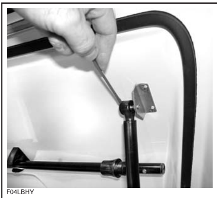
TYPICAL — LIFT TAB
