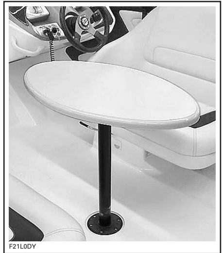
COCKPIT TABLE INSTALLED
