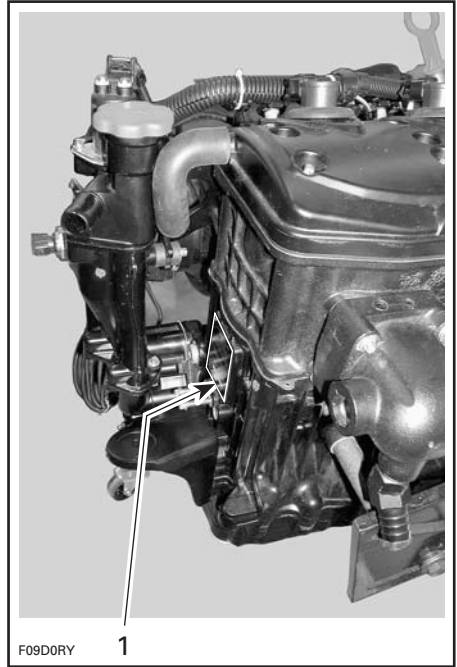
1. Engine Identification Number (E.I.N.)
