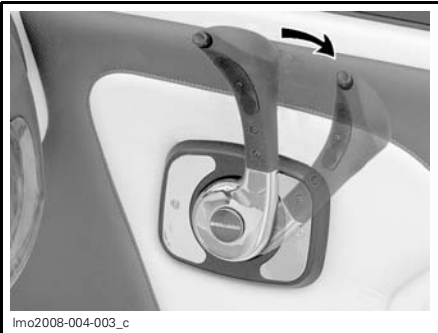
REVERSE FULL THROTTLE POSITION
