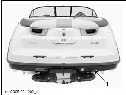
1. Hull Identification Number (H.I.N.)
