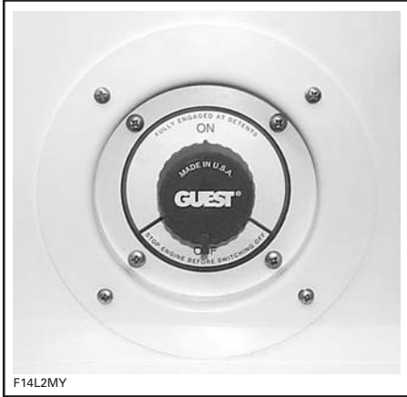
F14L2MY TYPICAL — MAIN BATTERY CUT-OFF SWITCH
