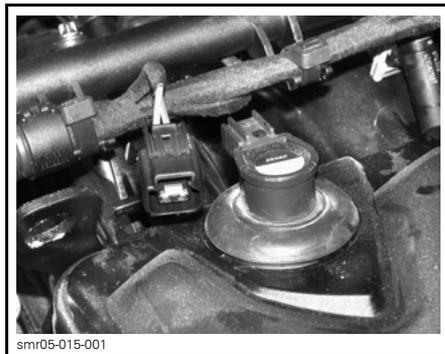
**DESCONECTE LOS CONECTORES DE LAS BOBINAS DE ENCENDIDO**
