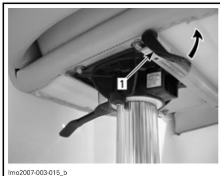
**TIRE DE LA PALANCA Y MANTÉNGALA EN LA PARTE DELANTERA DEL ASIENTO**
