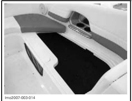
**STARBOARD SIDE — LIFT, THEN PULL SEAT CUSHION TO GAIN ACCESS TO THIS STORAGE COMPARTMENT**
