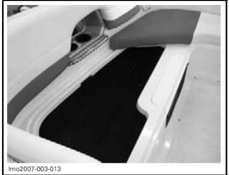
**PORT SIDE — LIFT, THEN PULL SEAT CUSHION TO GAIN ACCESS TO THIS STORAGE COMPARTMENT**
