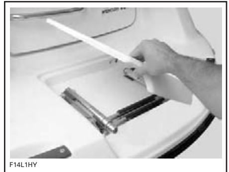
LIFT LADDER COVER UNTIL STOPPED BY RETAINING SPRING (SPRING NOT SHOWN)
