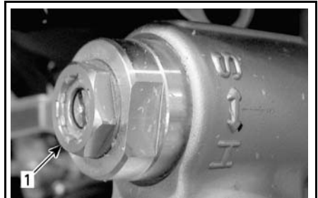
TYPICAL — REAR PRELOAD ADJUSTMENT A. Same length
