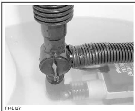
**METTRE LA SOUPAPE DANS CETTE POSITION, PUIS REMETTRE LE COUVERCLE EN PLACE**
