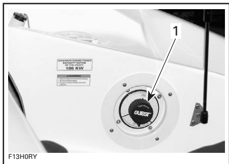
1. Main battery cut-off switch
