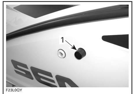
1. Fuel tank vent
