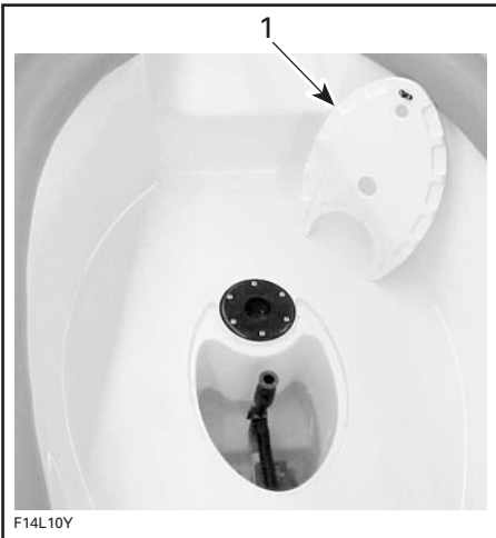
REMOVE FOUNTAIN SUMP COVER
