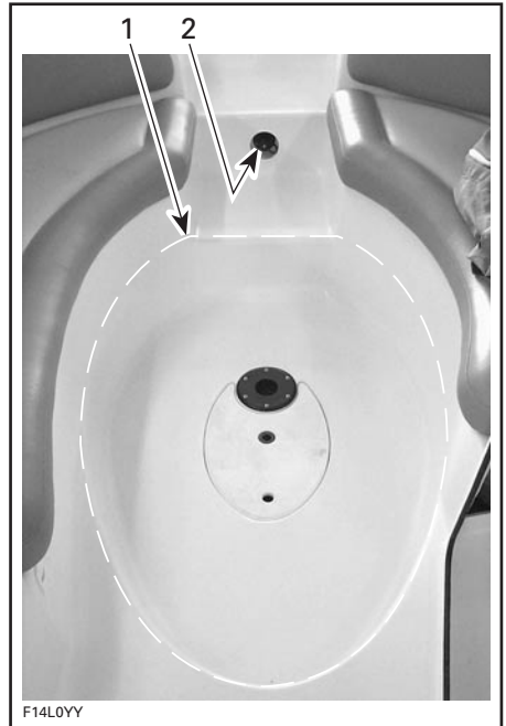
1. Foot well surface 2. Wash down valve
