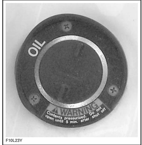
To add injection oil in the reservoir, unscrew the cap counterclockwise.
