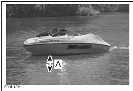
A. 90 cm (3 ft) of water under the hull
