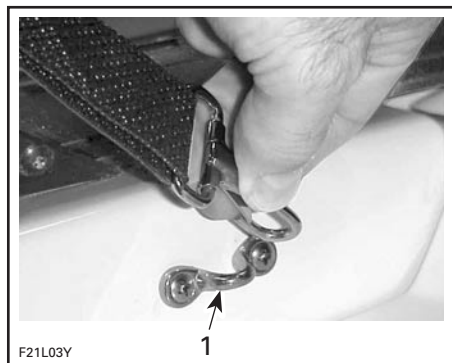
1. Hook strap to body eyelet
