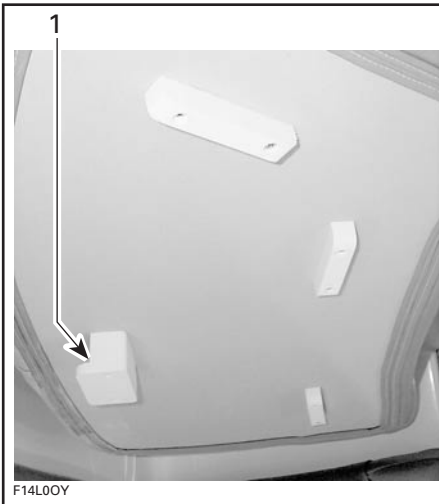
1. Position L-bracket first
