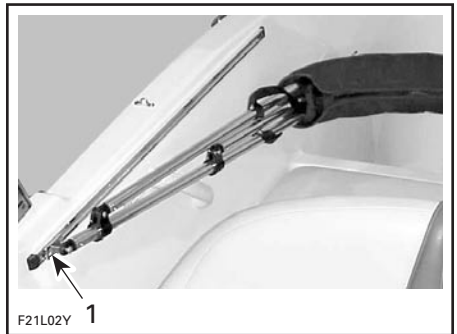
1. Bimini pivot base pulled forward on rail
