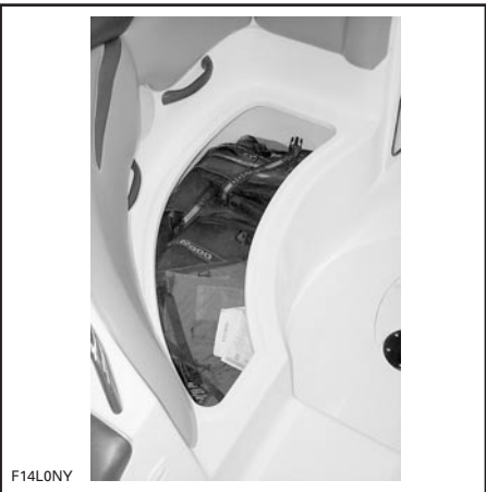
F14L0NY STARBOARD SIDE — LIFT THE PULL SEAT TO GAIN ACCESS TO THIS STORAGE COMPARTMENT
