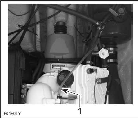
1. Pour antifreeze until it flows in bleed hose
