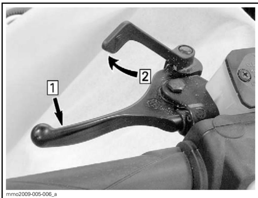
**TYPICAL — ENGAGE MECHANISM**
