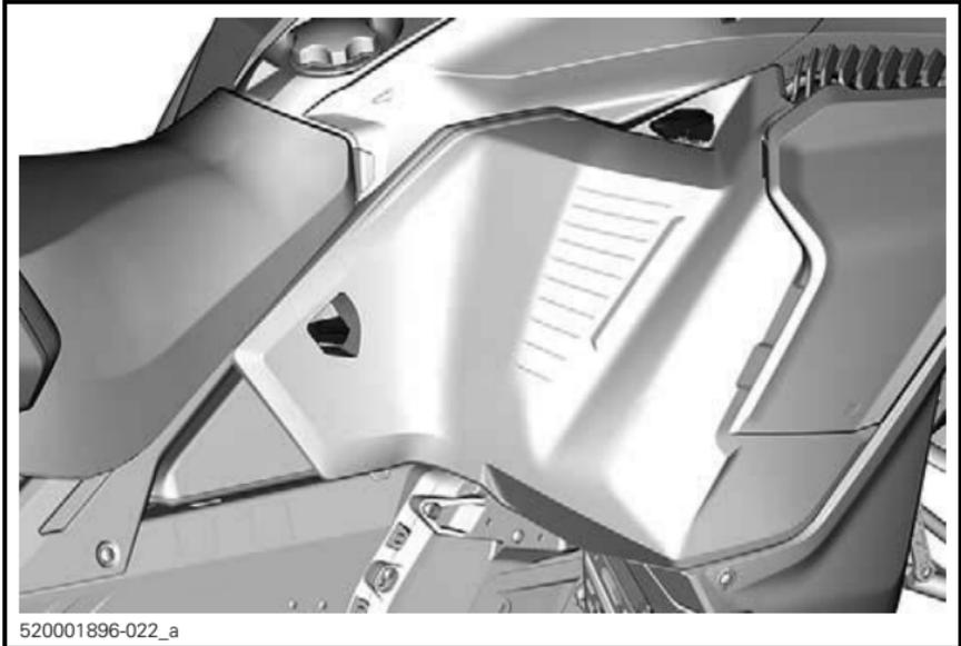
When closing panel, make sure latches are locked securely.
