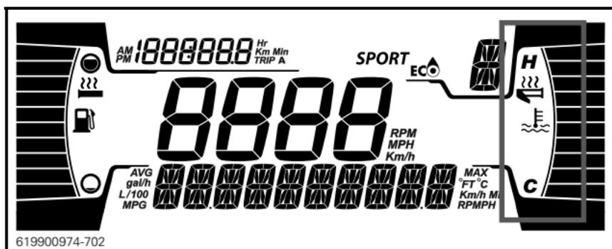
HEATED THROTTLE LEVER DISPLAY
