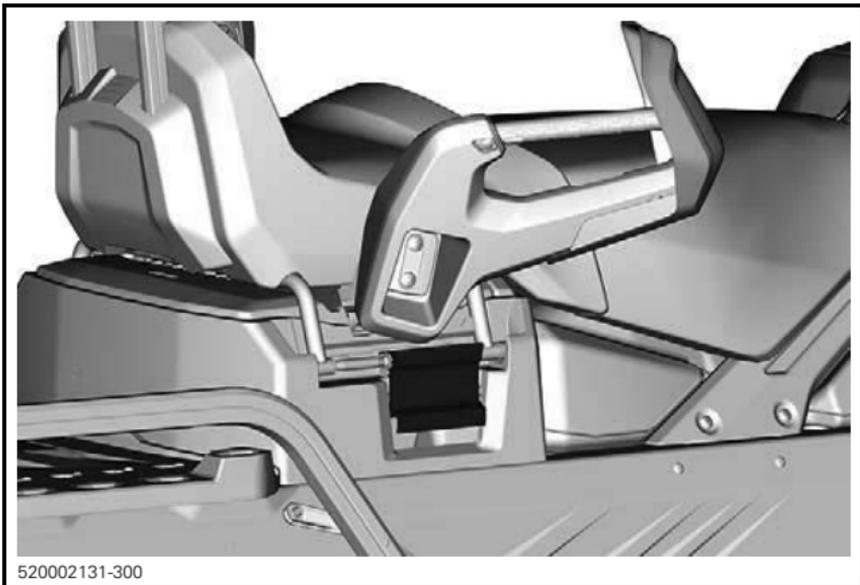
2. Lift the seat to disconnect the electrical connector.
