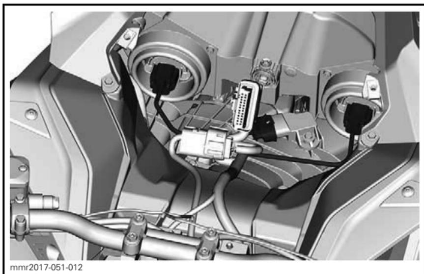
8. Loosen the air intake duct clamp.
