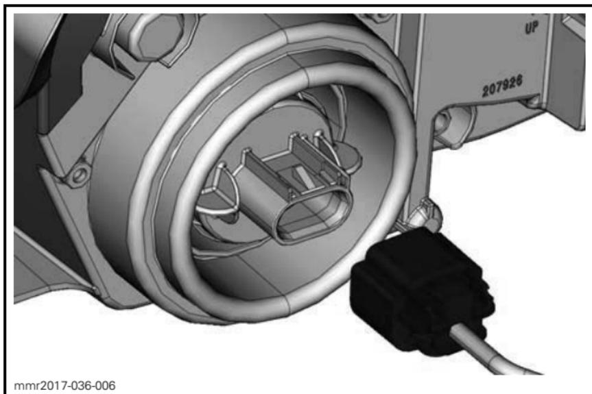
8. Unlock bulb by turning it counterclockwise.
