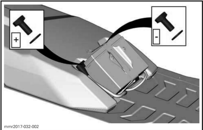
4. Remove battery hold down bracket.
