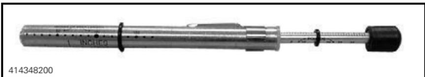
5. Set deflection between 40 mm to 50 mm (1.575 in to 1.969 in) using bottom O-ring.
