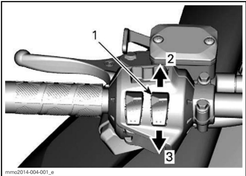
1. Heated throttle lever switch
