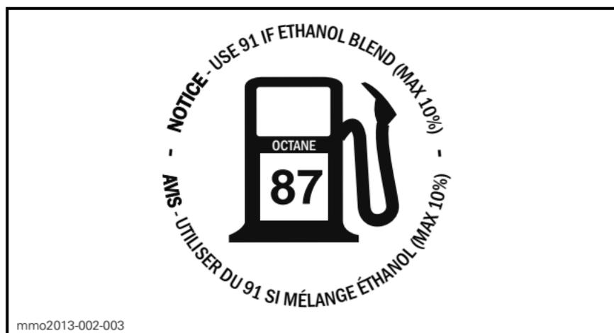
LOCATED ON FUEL CAP - ON 600 EFI ENGINE (IN COUNTRIES USING PUMP POSTED AKI (RON+MON)/2 OCTANE RATINGS)
