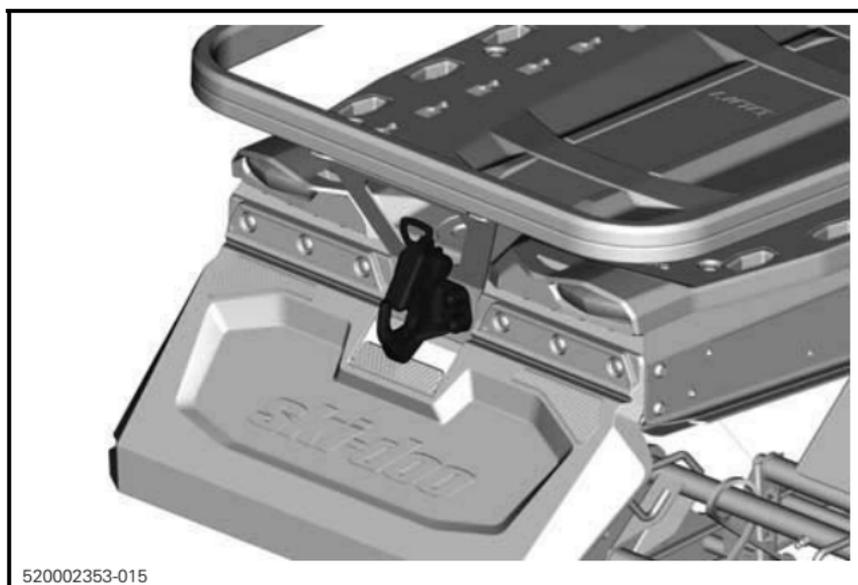
To open the hook, push and turn the handle to retract locking plate.
