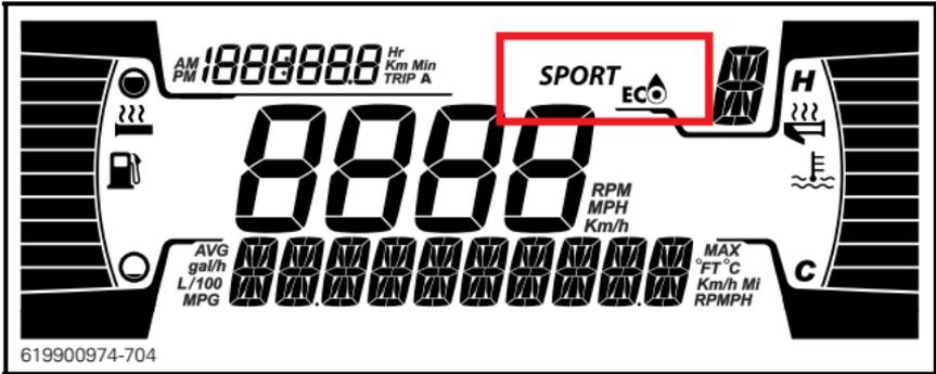
The MODE display indicates the selected mode of operation:
