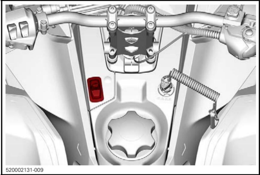
To activate Standard mode when in Sport mode, press bottom end of switch once.
