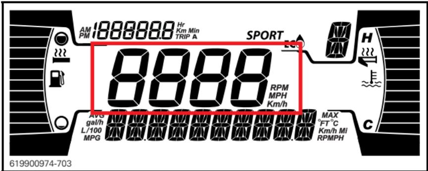
Display the RPM of engine or vehicle speed in Km/h or MPH.
