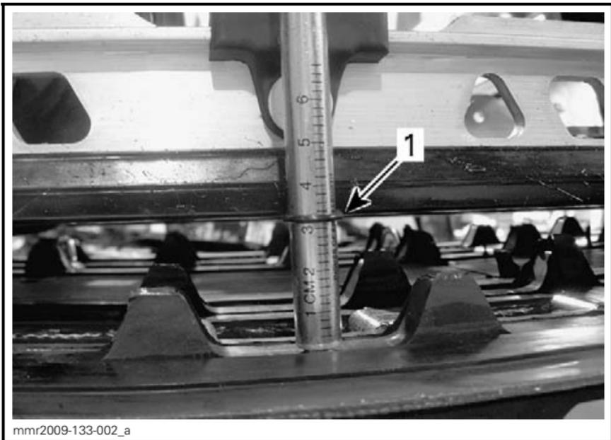
1. Deflection O-ring aligned with slider shoe
