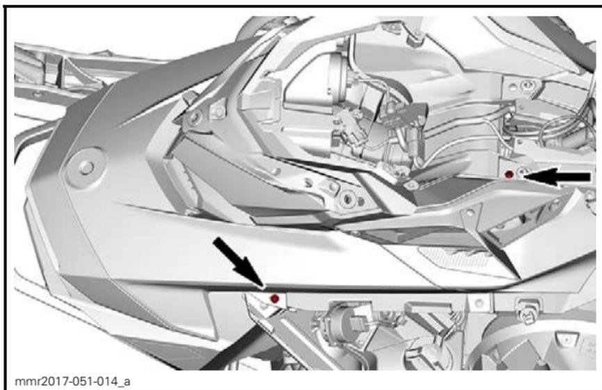
10. Free the rear end hooks of the upper body module from the slots in the console.
