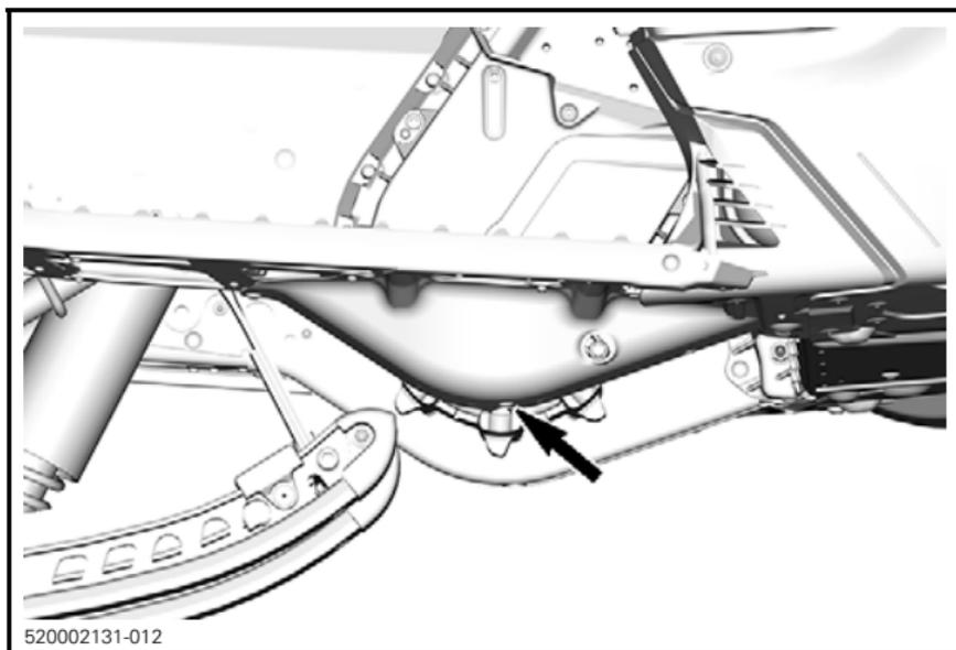
5. Wait a while to allow all oil to drain out of gearbox.
