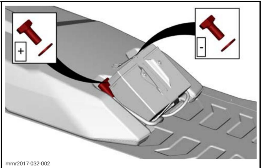
4. Remove battery hold down bracket.
