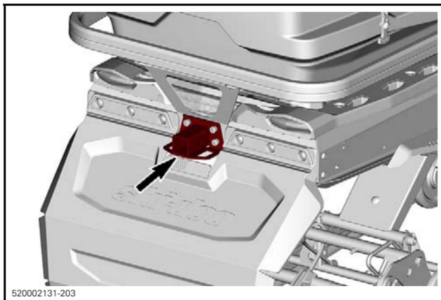
Use the hitch in conjunction with a tow bar to tow an accessory.
