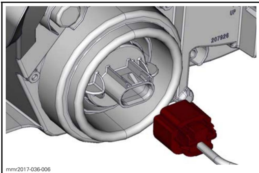
8. Unlock bulb by turning it counterclockwise.
