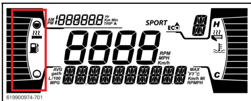
Heated grips will be in OFF position when there are no bars displayed on the gauge.
