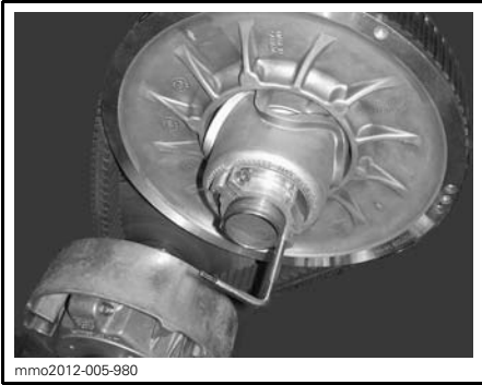
mmo2012-005-980 PULLEY EXPANDER INSTALLED ON ADJUSTER HUB
