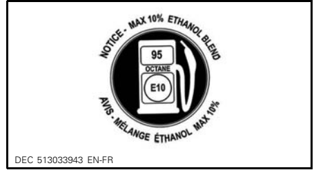
LOCATED ON FUEL CAP - ON 600 HO E-TEC ENGINE (IN COUNTRIES USING RON OCTANE RATINGS)
